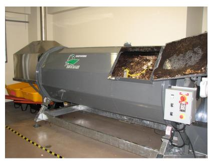
*Figure 5-1: Example of a Brome Composter (used for ICIC)*
